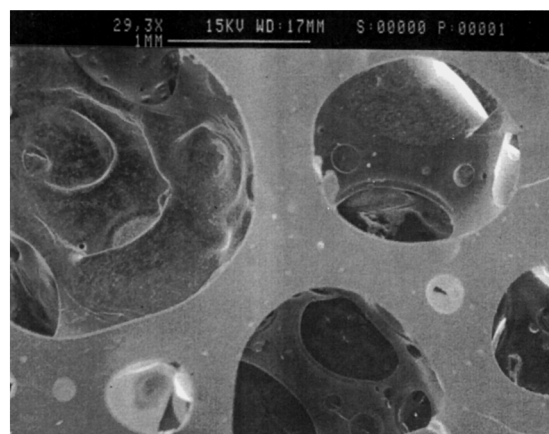
Figure 18 SEM of material produced using 3% Fluorad FC-430 fluorochemical surfactant and 97% TMPTA.
